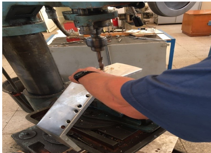
Figure 4.5 drilling the bigger holes using the drilling machine
