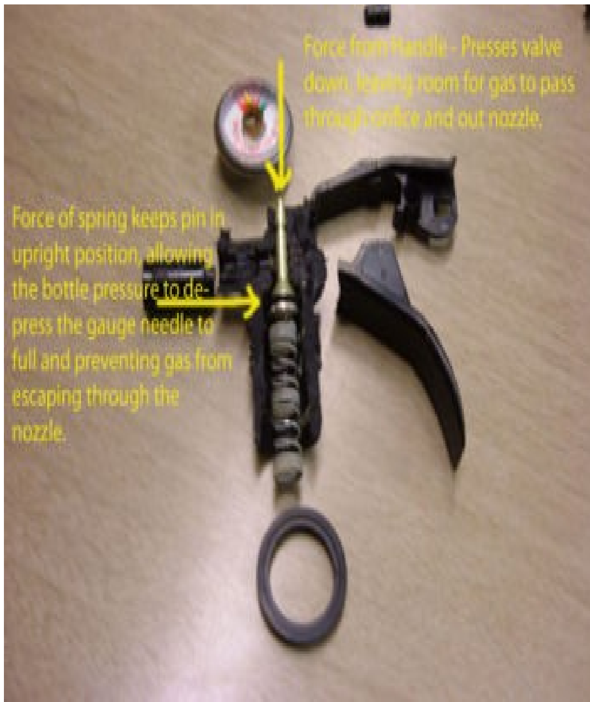
Appendix C3- Dissected fire extinguisher head showing the valve stem
